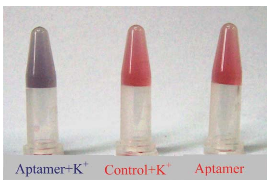
Fig. 2 Colorimetric detection of K^+ -induced structural variation of the K^+ aptamer. Four microliters of DNA solutions (8.3 \mu M), either in the presence or in the absence of K^+ (1.67 mM), were mixed with 200 \mu L of gold nanoparticles. The solutions were allowed to react for 4 min at room temperature and then 35 \mu L of buffered salt (10 mM phosphate, 0.5 M NaCl, pH 7.4) were added to each solution. From left to right: K^+ aptamer + K^+ ; control DNA + K^+ ; K^+ aptamer.
